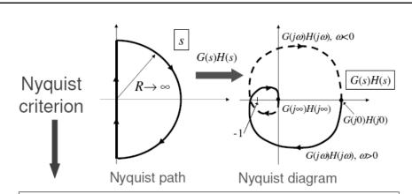
The Nyquist path is shown in the left figure. This path is mapped through the open-loop function G(s)H(s) into the Nyquist diagram, as illustrated in the right figure. Then
